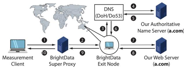
**Figure 1: Our Experimental Setup**—The measurement client, web server, and authoritative name server are under our control. We use proxy service BrightData to reach a large number of clients (exit nodes) located in different countries. Each client sends queries over DNS-over-HTTPS (DoH) and conventional DNS (Do53), and we measure the timing and results.
