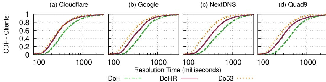
**Figure 4: Resolution Times by Resolver**—We show the distribution of resolution times for each public DoH resolver, both for the initial (*DoH1*) and repeated (*DoHR*) requests, along with the default (*Do53*) distribution for reference. Cloudflare stands out, as its *DoHR* resolution times very closely track *Do53* times for most clients.
