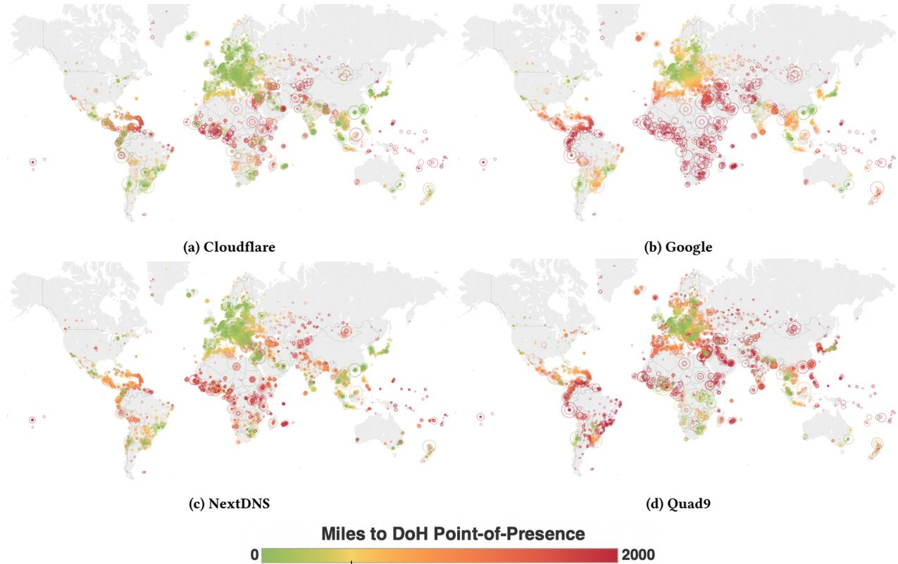
**Figure 9: Per-Client Distance to Servicing DoH PoP**—For each resolver, we present the distance for each client to the PoP that was used to perform the resolution. Providers excel in varying regions. Quad9, for example, assigns PoPs which are relatively close for clients in the southern part of Africa, but seems to underperform other providers by this metric in southern Brazil and Argentina.
