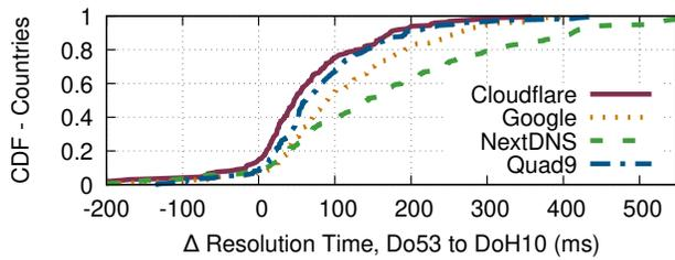
**Figure 7: DNS Performance by DoH Resolver**—We show the change in resolution times when switching from *Do53* to *DoH10*. The change differs significantly across DoH providers, with Cloudflare causing a slowdown of 49.65ms in the median case, while NextDNS causes a significantly greater slowdown of 159.62ms.
