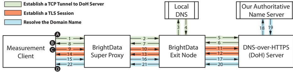
**Figure 2: DNS-over-HTTPS (DoH) Request Timeline**—Our measurement client sends a DoH request to the BrightData SuperProxy, which forwards the request to an exit node. The exit node then sends a DoH request to an DoH provider (e.g., Cloudflare), which resolves the domain name by contacting our authoritative name server.
